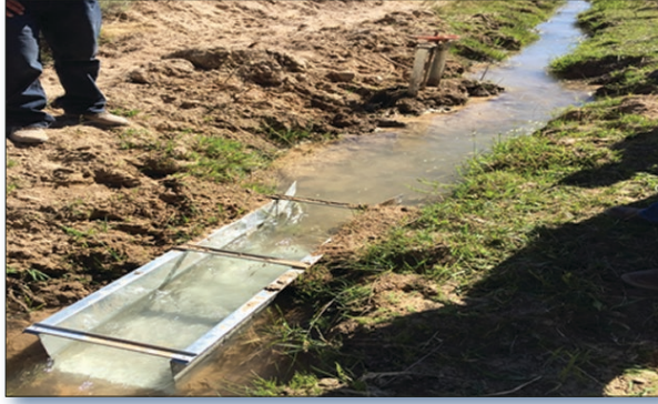
Figure 2. A flow measurement device was added to this irrigation diversion.
